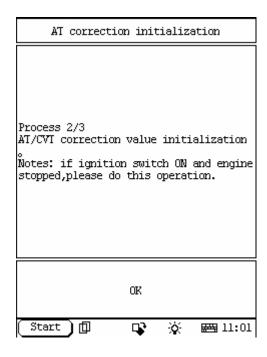
After confirming this operation, the screen will display Process 2/3 Menu: AT correction initialization. Note: please do this operation with ignition switch ON, and engine OFF.
