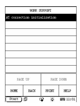
After selecting AT CORRECTION INITIALIZATION MENU, the screen will display the Process 1/3 Menu. It will prompt you that: If you want to change AT, CVT or ECU, please do this operation. Press 'YES' to do this operation. Press [NO] to exit.
