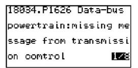
As seen on the left bottom, the front digit is the No. of the displayed fault code, while latter digit is the number of total fault codes.
