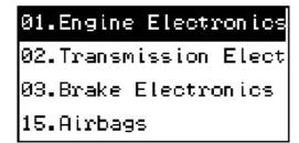
There are 78 systems available. Here let's take [01. Engine Electronics] for example. Select [01. Engine Electronics], and press [←] key. The screen will display the following message:
