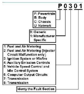
A typical DTC is shown above. It consists of five characters: four digits proceeded by one letter. The first letter indicates the main system where the fault is located (Powertrain, Body, Chassis or Network). The second character is a number and it identifies whether the code is an SAE standard code (Generic) or manufacture specific code. The remaining three numbers provide information regarding the sub-system and section that are malfunctioning.
