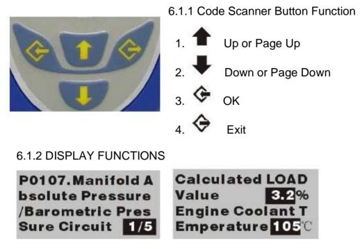
The graphic LCD can display graphics and letter in lattice 128x64. The DTC and
