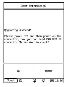
6. Check the version again. If the current version is the same with the downloaded version, it says that update successful; if not, please check CAN BUS II adaptor, main cable and the connection between main cable and X431. And do operation from step 2 to step 6 again.
