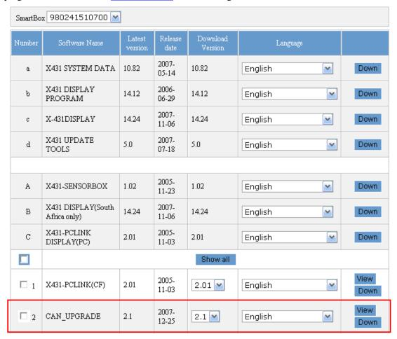
Registered user can down the update program from the website. The way for CAN BUS II update is similar to that of diagnostic software. Updated CAN BUS II adapter can be compatible with more models.
